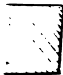
STEEL ROUGH OR IRREGULAR
